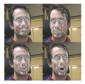
Figure 4: Automatic face and facial feature tracking. The simple face model adapts to each frame in the sequence (every tenth frame shown), and MPEG-4 FAPs can then be extracted from the model.
