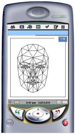
Figure 4: The Facial Animation Player early prototype implementation on Symbian Quartz using the Candide face model from Linköping University.
