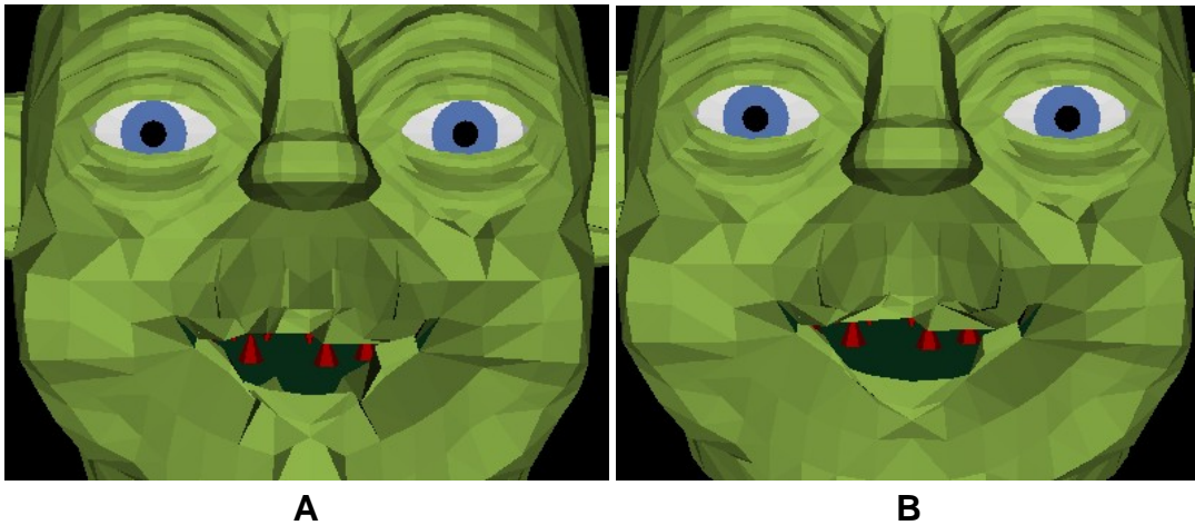
Figure 8: A: Aliasing artifacts clearly visible on lower lip. B: When filtering is applied, lower lip is smooth.
