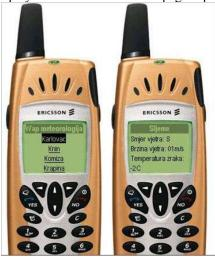
Figure 11. Mini client display: WML
